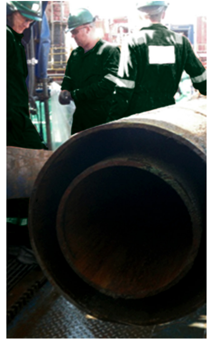
Successful cut 13 3 / 8 -in. and 20-in. dual-casing strings at surface.
