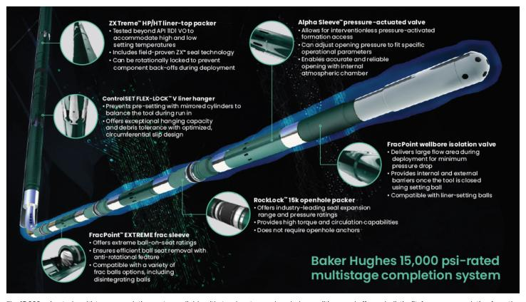
The 15,000 psi-rated multistage completion system reliably withstands extreme downhole conditions and offers a holistic, fit-for-purpose solution from the liner top to the toe of the well, eliminating the complexity of building a solution assembled by multiple vendors.
