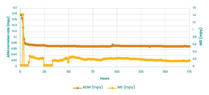
Corrosion rates were monitored both during and post passivation. Baker Hughes's recommendation of CES filtration equipment combined with the **LIFESHIELD inhibitor** program allowed the refiner to realize an ROI of 412%.
