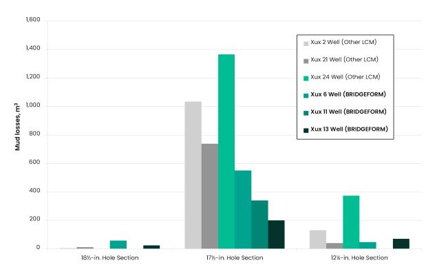
BRIDGEFORM saved the operator approximately \$2 million USD due to reduced mud losses and increased efficiencies.
