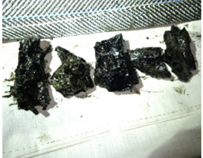
Small pieces of rubber and fiber flakes retrieved in the third run prompted the Baker Hughes team to perform a dummy run to determine if ID was free from debris and ready for the upper completion stabbing.
