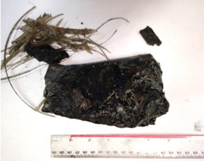
In the second run, larger rubber pieces (up to 6 in.) were pulled from the PBR via the VACS G2 system.
