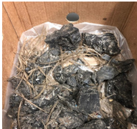
Retrieved pieces of rubber and fiber flakes from the first run proved ID of PBR clogged with debris.
