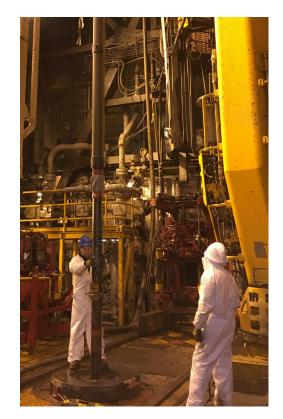
The GeoFORM system is run downhole like a sand screen—but can be installed by a two person crew, and doesn't require special pumping equipment or proppant, making it ideal for remote locations. The GeoFORM system saved five days of rig time in this challenging openhole lateral.
