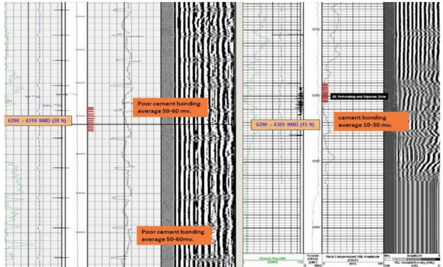
Left—CBL/VDL indicates poor cement bond/free pipe prior the squeeze cement job. Right—CBL/VDL indicates zonal isolation after the squeeze cement job using the SealBond cement spacer system.
