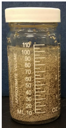
Left, the Stimforce III vessel ready to sail; right, results of Diamond PAQ HT sand settling tests performed at 176° F (80° C) for 60 minutes
