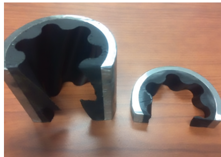
The stator elastomer in the Versa-Drive Ultra workover motor showed minimal wear.
