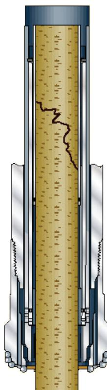
Freed inner sleeve telescopes up core barrel; second sleeve receives new core.
