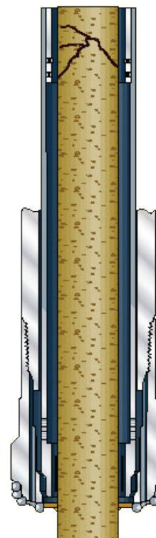
Second jam releases second telescoping inner sleeve. Coring continues until third jam occurs.
