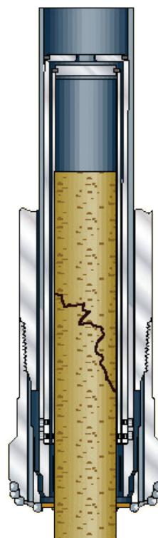
First jam enters sleeves and shears the pins.
