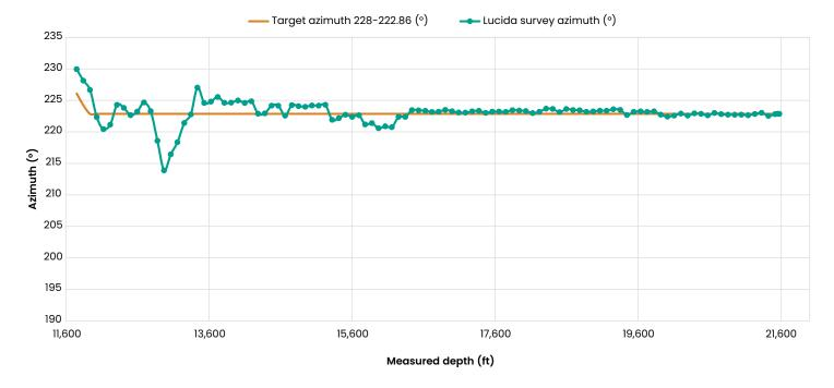
Automated wellpath trajectory control system delivers tight azimuth control.
