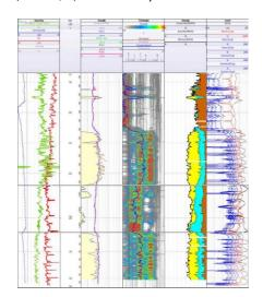
The MagTrak service acquires high-quality pore space measurements while drilling without impacting rates of penetraion (ROP), and includes accurate porosity, fluid type identification, and an estimate of permeability.
