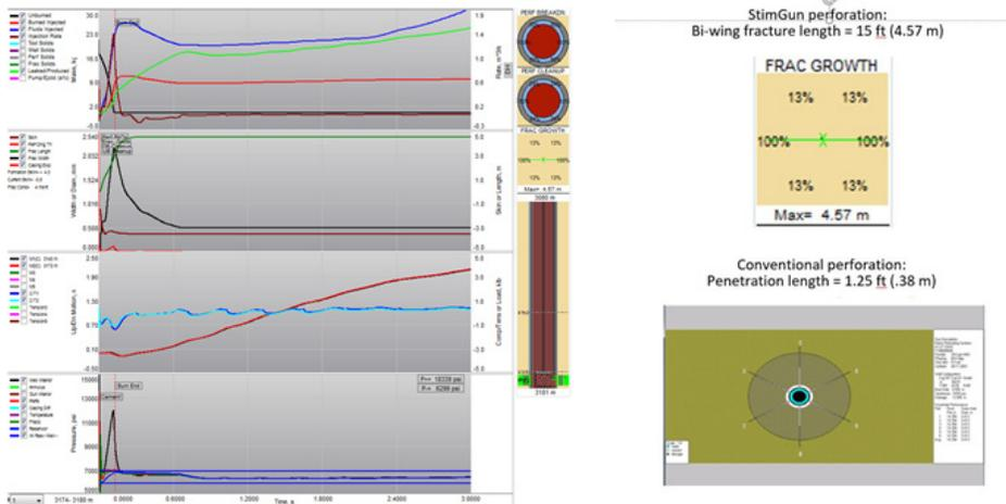
An operator in south India was facing production issues in an exploratory gas well. The company was trying to evaluate the producibility of the formation which had near-wellbore formation damage from drilling, completions, and perforating activities. In addition, the low native permeability of the formation (10% porosity and 1-4 mD permeability) had led to greater formation loss and permeability in the damage zone.
