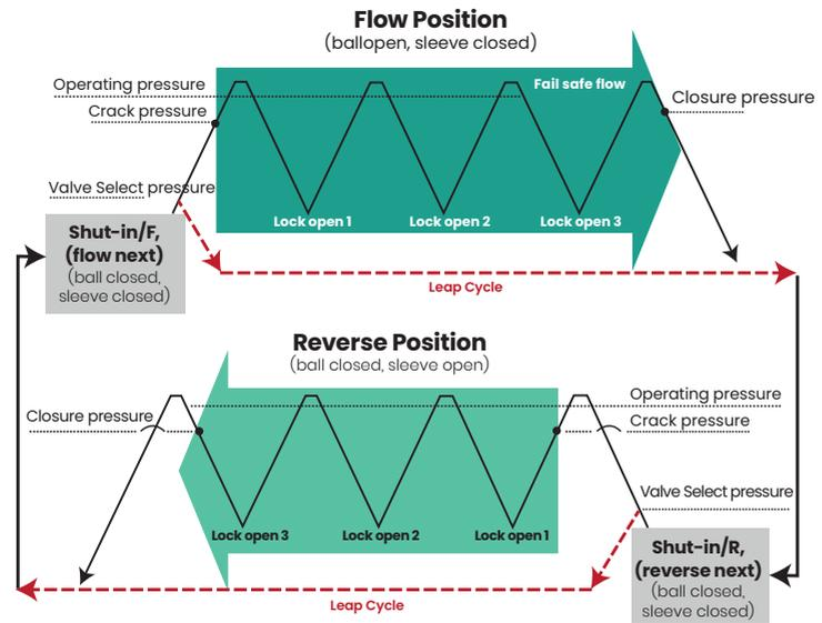
The sequencing interlock enables ball or circulation valve reset without having to repeat the entire valve sequence.
