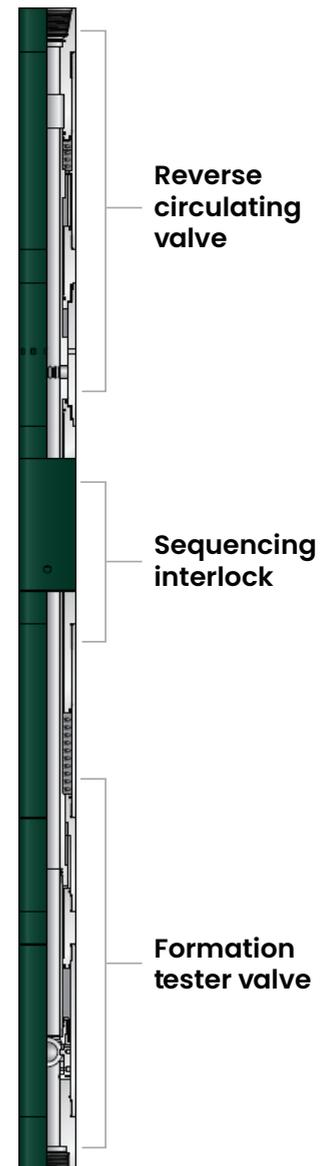
The xDCV combines the shut-in and circulating valves into one flexible tool.
