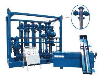
the HPDUs in 15 filtration cycles. A total of 100.5 lb (45.5 kg) of solids were removed. The HPDU on the boost line processed 7,914 bbl, capturing 11 lb (4.9 kg) of solids. The HPDU at the standpipe processed 48,119 bbl, capturing 89.5 lb (40.6 kg) of solids.
