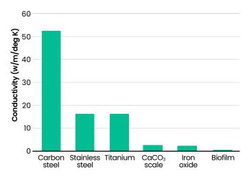
W.G. Chiracklis, Microbial biofouling control, in: Biofilms, W.G. Chiracklis and K.C. Marshal (eds.), Wiley Interscience, Toronto, 1990; pp. 585-633. Biofilms dramatically reduce heat-exchange capacity.
