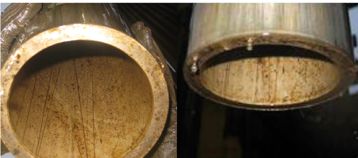
Tubing after being pulled to surface.
