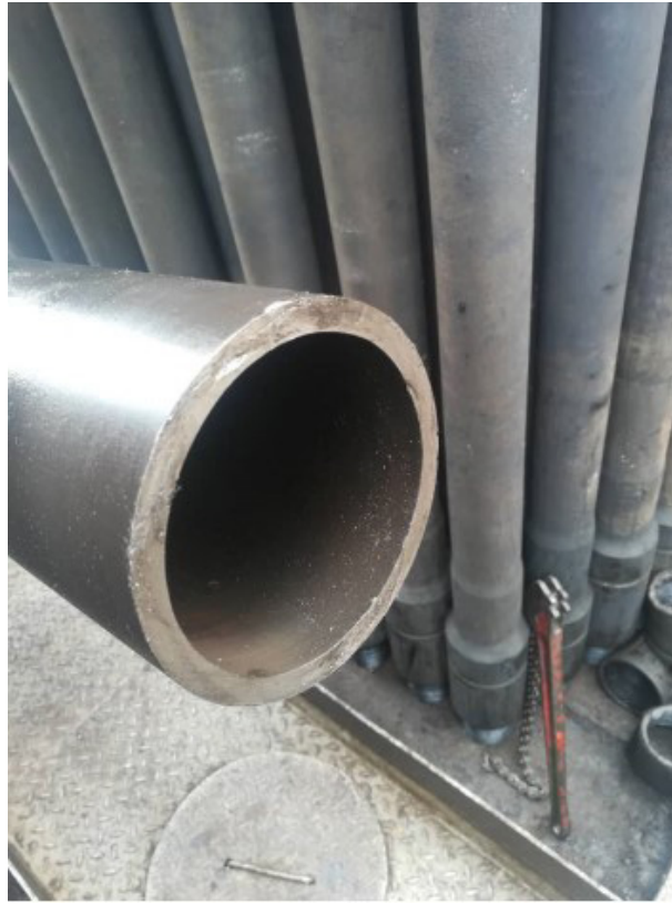
The first image shows the failed pipe cut attempted by another wireline company; the second image shows the precise cut made by the Baker Hughes MPC
