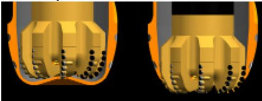
This illustration shows the mechanics of the EZReam shoe drillout with a standard PDC bit. The unique concave profile ensures EZReam shoes are drilled out from the center to the shoulder, eliminating the risk of undrilled junk left in the hole bottom.
