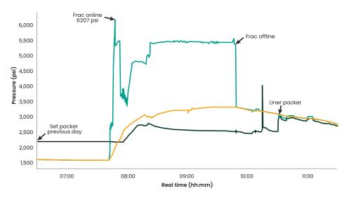
Recorded data from memory gauges during the refracture treatment. Green is the injection pressure into the formation. Dark green is below the packers. Orange is above the packers.
