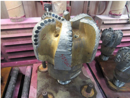
Bit body shows no sign of damage and cutting structure shows minimal wear.
