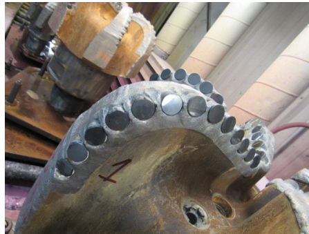
Cutting structure shows minimal wear, proving the bit can drill faster and farther than competitors' offerings.
