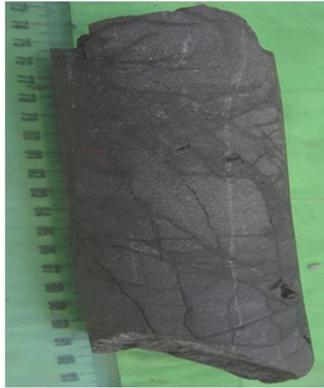
Fractures detected in wellbore image data are verified against recovered core.
