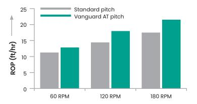
Two bits, differing only in cutter arrangements, were run in Carthage limestone at three different revolutions per minute (RPMs). At all speeds, the Vanguard bit, with computer-modeled cutter arrangements, consistently drilled at a higher ROP.
