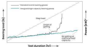
During a laboratory test, a bearing with standard lubrication initially seized after 23 hours and completely failed in 30 hours. A bearing with the new Vanguard grease ran to the test machine limits, running long hours without signs of high torque or the onset of bearing failure.
