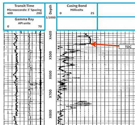
Fig. 1: Original 1979 CBL log shows TOC detected around X450 ft
