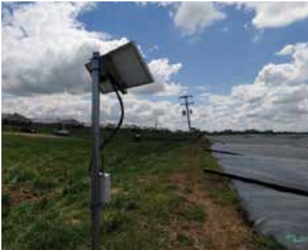
LUMEN Terrain sensor installed for continuous monitoring at perimeter of biogas lagoon.
