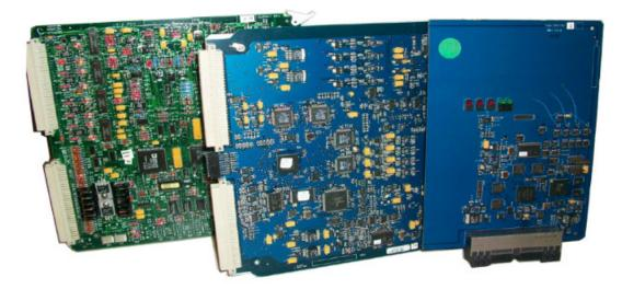
Throughout the late 1990's additional monitor cards were introduced expanding the application footprint of the 3500 system beyond solely vibration protection for turbo machinery. These expansions allowed for overspeed applications, temperature measurements, position measurements such as case expansion and thrust position, as well as the first local display option and additional communication gateway support to allow deeper DCS integration.
