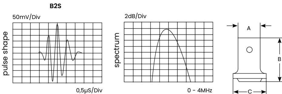
Typical waveform and frequency spectrum
