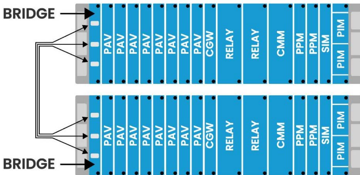
Figure 1: Rear View of Two Chassis Connected by a Bridge.
