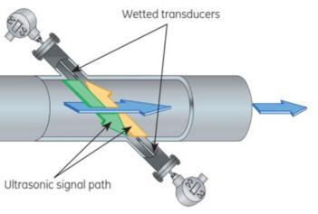
Figure #1: Ultrasonic Flow Meter Transit Time
