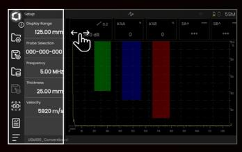
For the most important parameters, swipe right for the **sidebar**.
