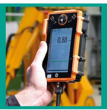
The Krautkrämer DMS Go+ offers a comprehensive handheld solution for thickness measurement, data recording, and data management in a wide range of applications and environments.
