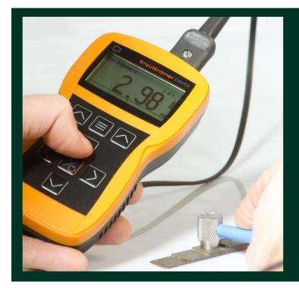
The Krautkrämer DM5E, also available in the Basic and DL version, represents the highest standard of portable corrosion monitoring thickness gauges.
