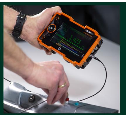
The Krautkrämer CL Go+ sets a new standard for precision thickness gauging, offering unparalleled accuracy and a user-friendly experience in a compact and durable design.
